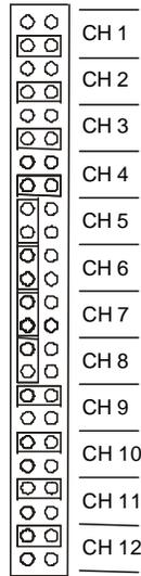
The jumper block indicates the correct jumper positions for the wiring shown.
