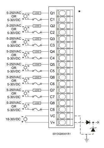
Warning: To protect the module and associated wiring from load faults, use external fuse (4 A) as shown. This warning affects DQM202, Revisions D or higher.
