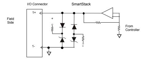
Specification for transient voltage suppressors (transorbs) used on output circuitry is 11 V, 600 W.
