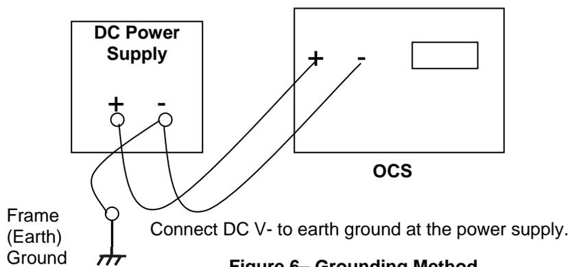
Figure 6– Grounding Method (OCS shown in this example.)
