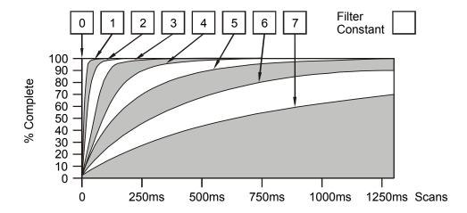
**Digital Filtering:** The illustration above demonstrates the effect of digital filtering (set with Filter Constant) on module response to an input change.
