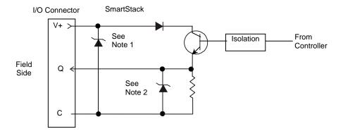
**Note 1:** Specification for transient voltage suppressors (transorbs) used on output circuitry is 54 V, 600 W.
