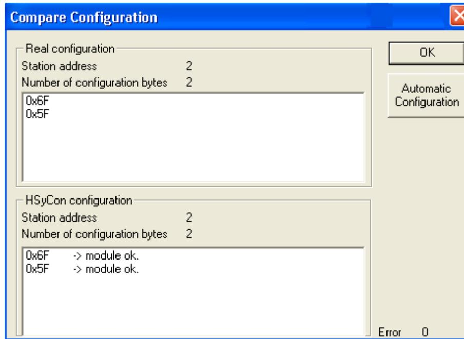
Figure 48: Online > Device Diagnostic > Compare Configuration
