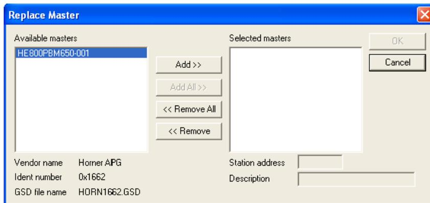
Select the required Master by clicking on it in the **Available Masters** list. Click the **Add** button to put the Master in the **Selected Masters** list. Confirm the selection by with **OK** and the Master will be replaced.
