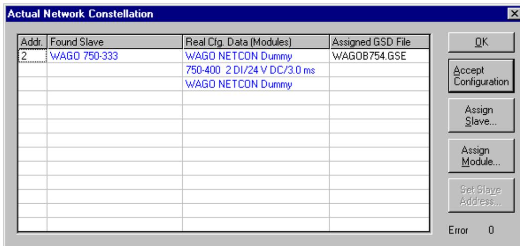
**Figure 38: Online > Automatic Network Scan - Example for Assignment**
