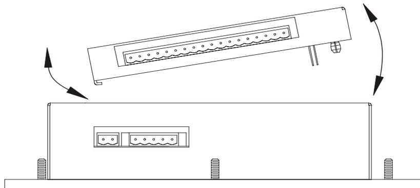
**Figure 1.1 – Installing a SmartStack Module in an OCS**
