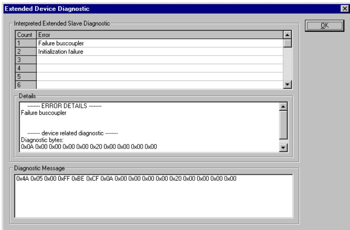
**Figure 49: Device Diagnostic (PROFIBUS-DP extended diagnostic)**
