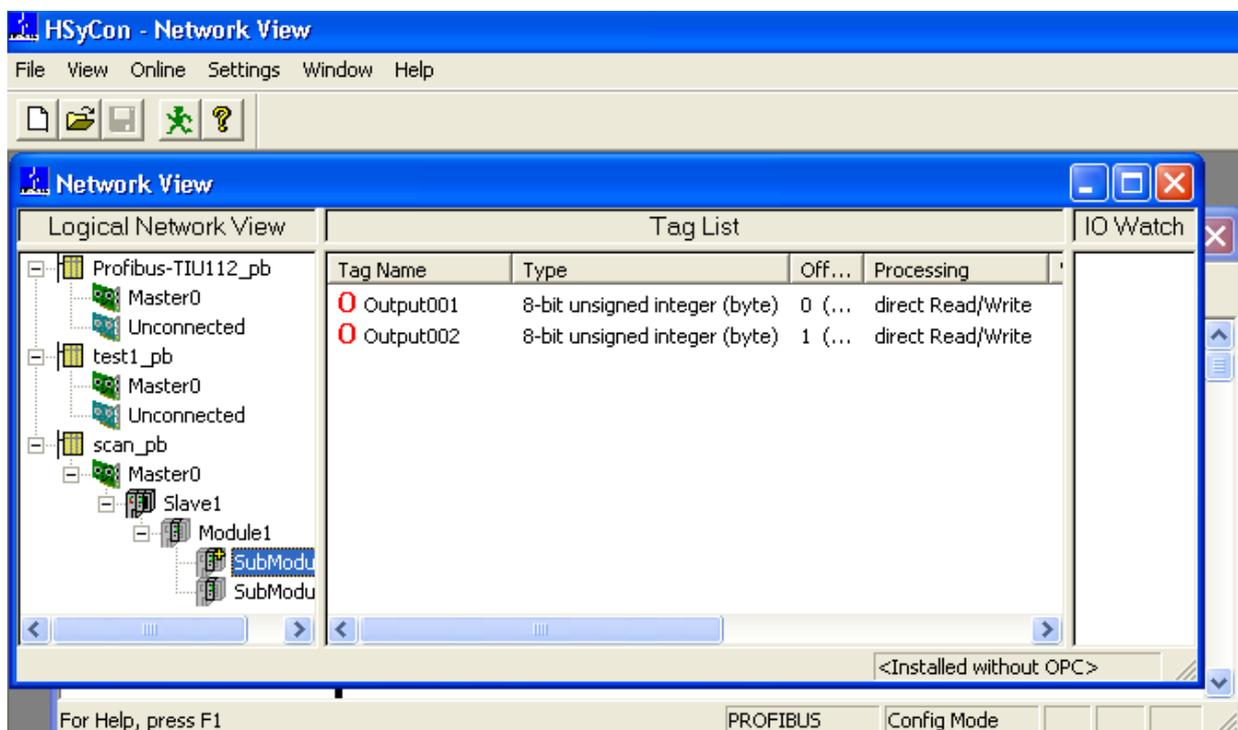
Left click on the module desired and the tags (I/Os) will be displayed in the centre window of the Logical Network View.
