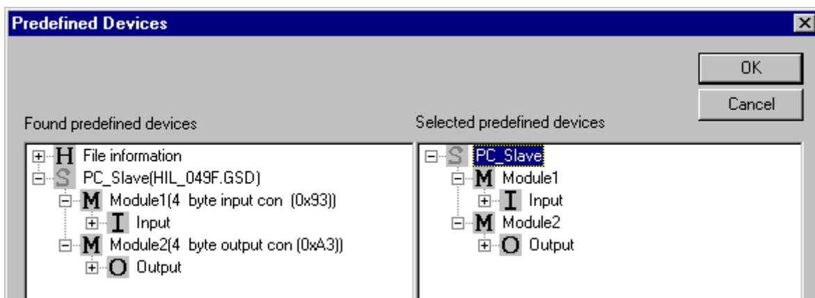
Figure 9: Inserting predefined device – PDD (3)
