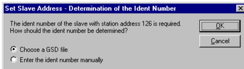
Figure 42: Online > Automatic Network Scan > Set Slave Address
