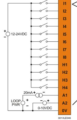
Note: Loop Power requirements are determined by the transmitter specification.
