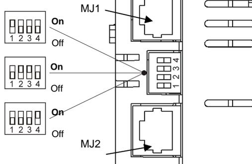
SW1 - ON enables **MJ2** RS485 port termination (121 Ohms). OFF disables **MJ2** RS485 port termination.
