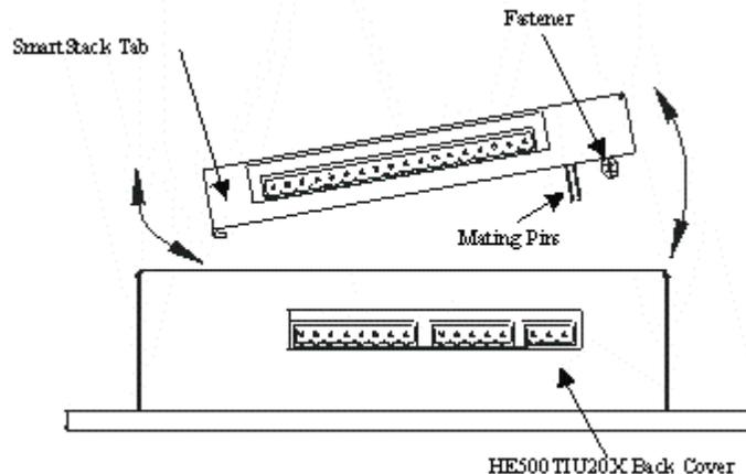
Figure 11.1 – Installing a SmartStack™ Module in a TIU.
