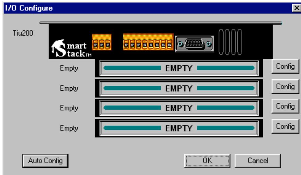
**Figure 11.1 – SmartStack Configuration**
