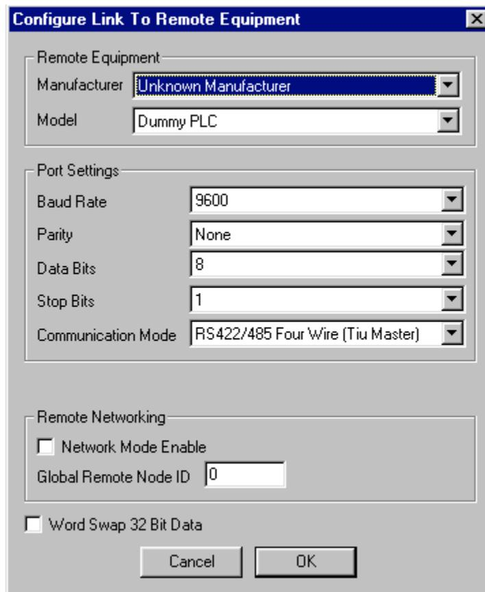
Figure 2.2 – AE Configuration Box
