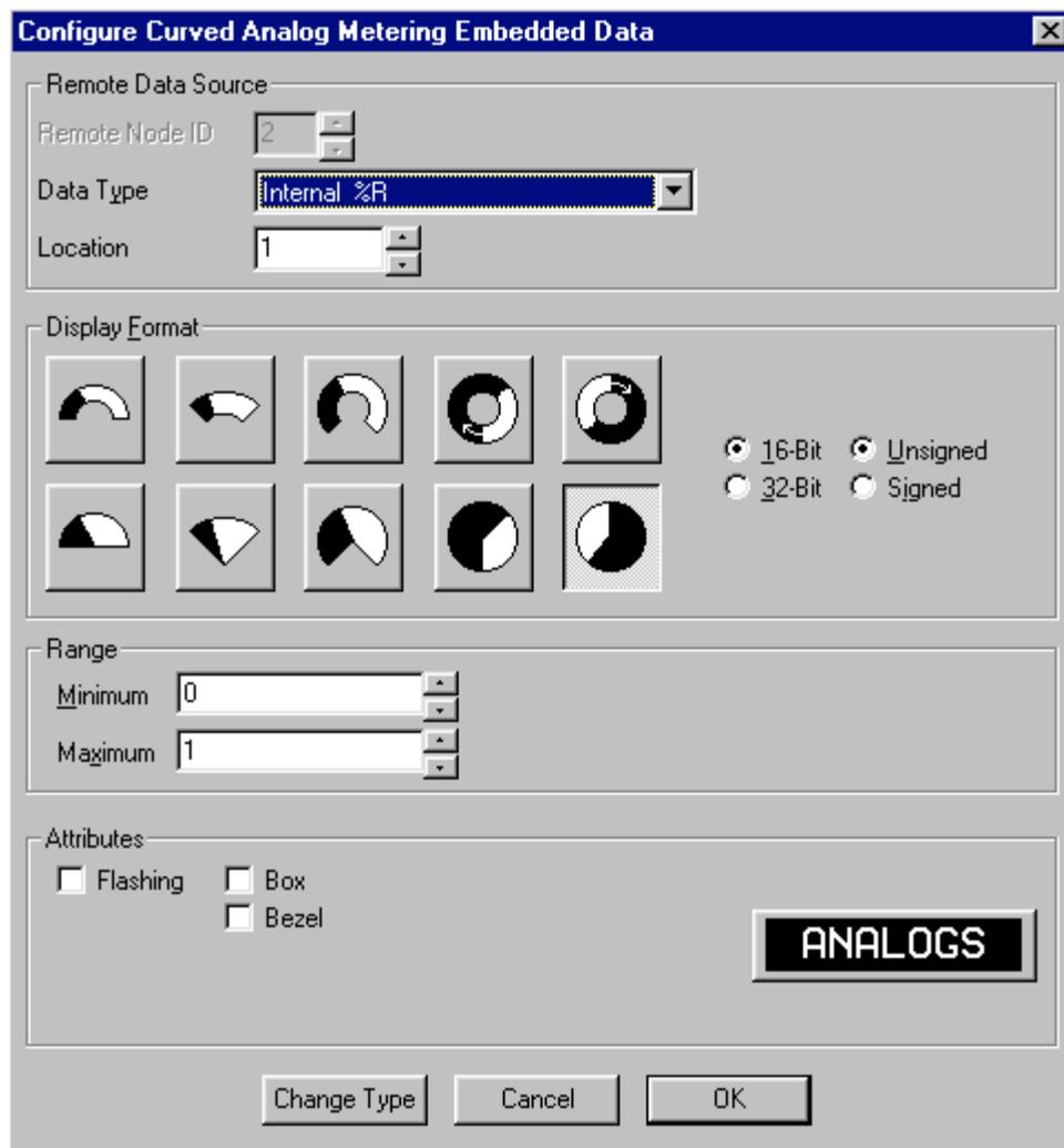
**Figure 8.18 - Configure Curved Analog Embedded Data****8.4.7.1 Remote Data Source**
