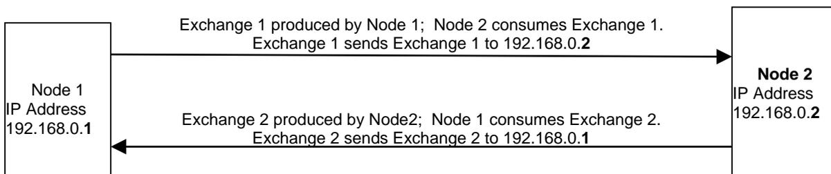
**Figure 17.6 Example of Exchange Interaction**
