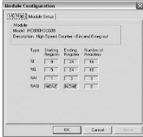
**Figure 6 - Example 1 - I/O Map for HSC in Second Slot**
