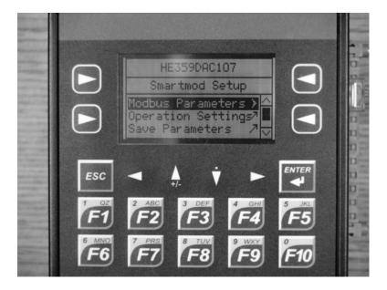
Note that the top line in this screen should accurately reflect the type of Smartmod connected, in this case a DAC107.
