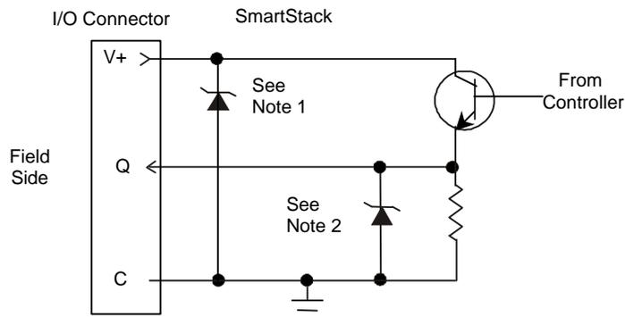
Note 1: Specification for transient voltage suppressors (transorbs) used on output circuitry is 36V, 300W.
