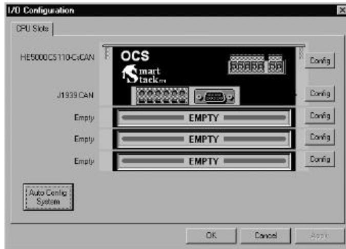
Figure 3.3 – JCM200 Module is Added
