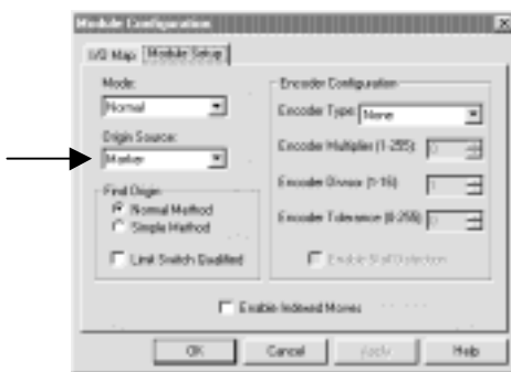
Figure 3.6 – Stepper Module Configuration Screen
