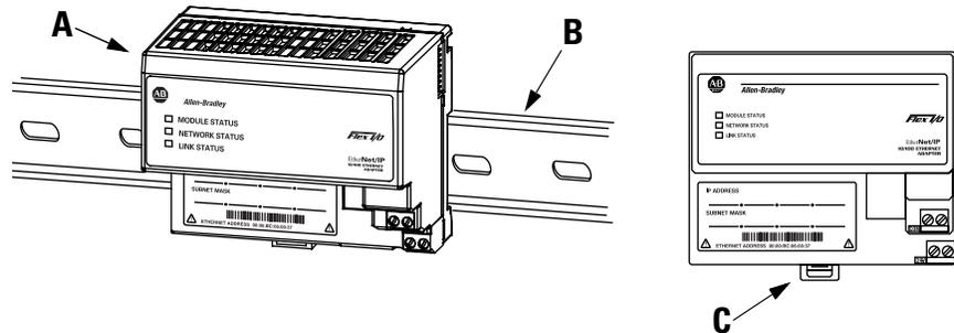
1. Position the EtherNet/IP adapter module (**A**) on a 35 x 7.5mm DIN rail (**B**) (A-B pt. no. 199-DR1; 46277-3; EN 50022) with the bottom rotated outward at a slight angle.
