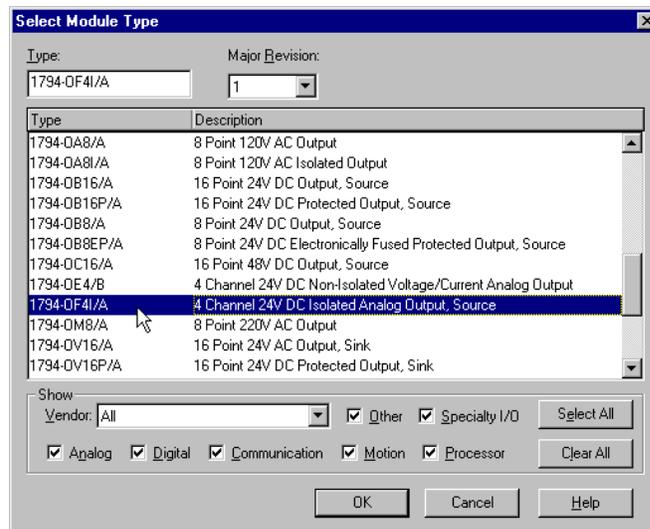
2. Select the **1794-OF41/A** analog output module from the list and click on **OK**.
