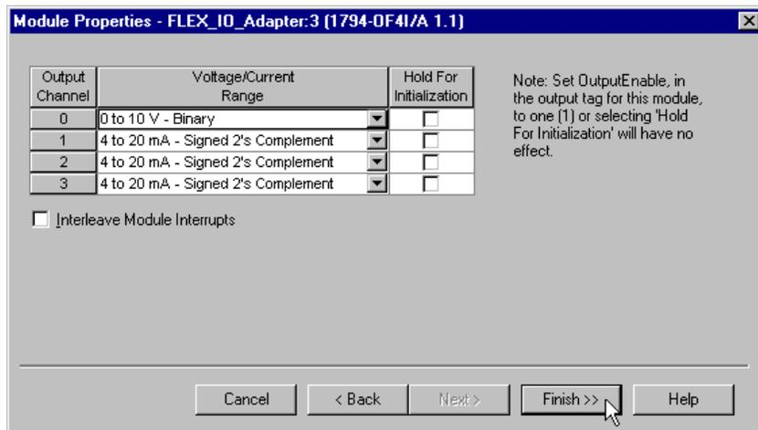
9. Use the pull-down list to set the **Voltage/Current Range** for **Channel 0** to “0 to 10V - Binary” to match the input configuration of the 1794-IF41 module. You can leave the other parameters at their default values.
