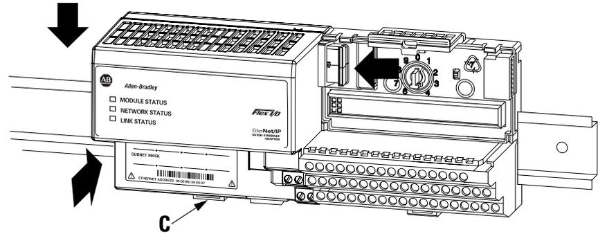
8. If the adapter module does not lock into place, use a screwdriver or similar device to pull locking tab **C** down while pressing the adapter module flush onto the DIN rail. Then release the locking tab to lock the adapter module in place. If necessary, push up on the locking tab to lock.
