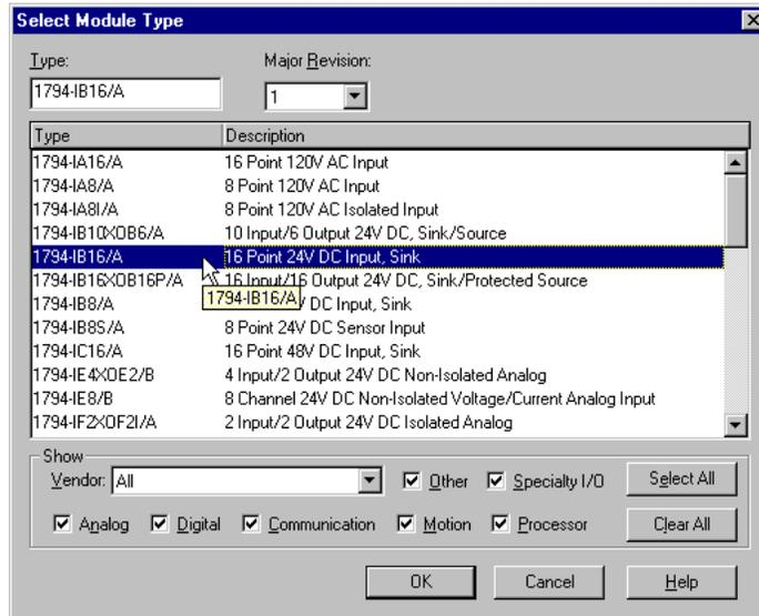
3. Select the **1794-IB16/A** digital input module from the list and click on **OK**. The **Module Properties** window will open.
