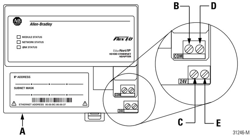
1. Connect the Ethernet network cable to the RJ-45 connector (A) on the underside of the adapter.
